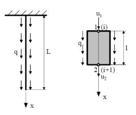
Finite element of tensile shaft.
