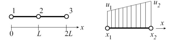
Figure 1.1: Two one-dimensional linear elements and function interpolation inside element.
