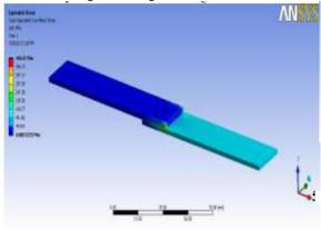
Fig 4.1.Vonmises stress of riveted joint
