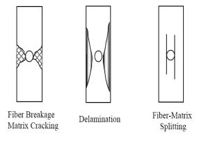
**Figure 2-3.** Typical tensile failure modes in composite laminates containing a circular hole.
